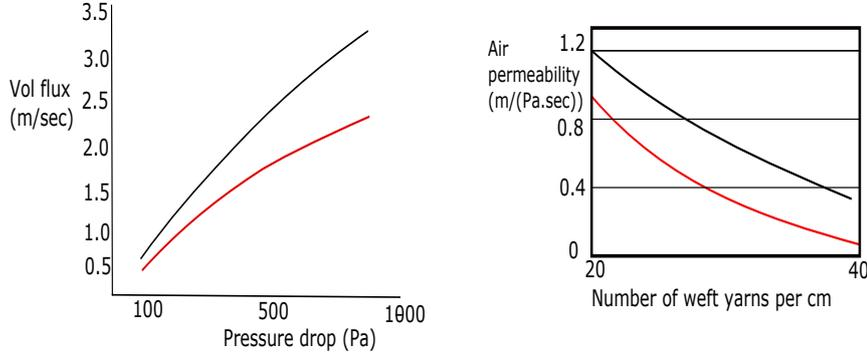
Figure 2. Air permeability data: *Left*: Volumetric flux (m/sec) of two non-weave sample fabrics as a function of pressure drop across the fabric. *Right*: Changes in the air permeability in a woven fabric due to weave spacing. The upper curve has a weft number of 60, the lower a weft number of 20. In both cases the warp number is 20 Nm, with the number of warp yarns per cm: 20; data taken from Ogulata [6].
