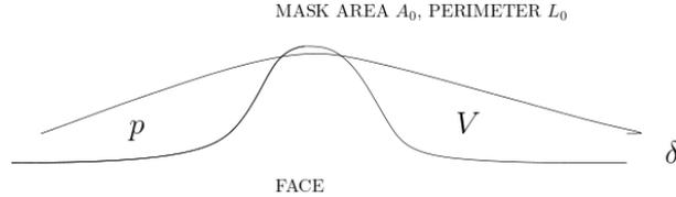
Figure 1. Mask geometry: The mask (area  $A_0$ ) fits onto the face. The volume of air between the face and the mask is  $V$ . The pressure within this space above atmospheric pressure is  $p$ . The effect of a sneeze or cough will be to increase  $p$  and  $V$ . The effective spacing around the edge of the mask with perimeter  $L_0$  is  $\delta$ .
